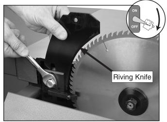
Figure 31. Installing the riving knife.
